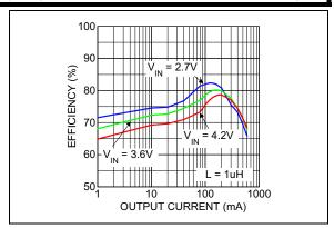
**FIGURE 2-4:** Efficiency  $(V_{OUT} = 1.0V)$ .
