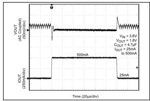
FIGURE 2-22: Load Transient, (25 mA to 500 mA).
