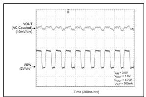
**FIGURE 2-18:** Switching Waveforms,  $(I_{OUT} = 500 \text{ mA}).$
