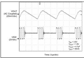
**FIGURE 2-15:** Switching Waveforms,  $(I_{OUT} = 5 \text{ mA}).$
