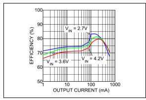
**FIGURE 2-3:** Efficiency  $(V_{OUT} = 1.2V)$ .
