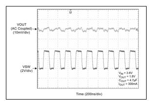
**FIGURE 2-17:** Switching Waveforms,  $(I_{OUT} = 300 \text{ mA}).$
