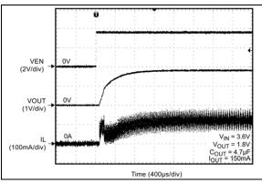
**FIGURE 2-21:** Start-Up,  $(I_{OUT} = 150 \text{ mA})$ .
