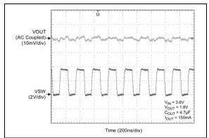
**FIGURE 2-16:** Switching Waveforms,  $(I_{OUT} = 150 \text{ mA}).$
