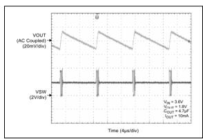
**FIGURE 2-14:** Switching Waveforms,  $(I_{OUT} = 10 \text{ mA}).$
