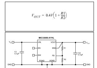
FIGURE 4-1: MIC33050-AYHL Application Schematic.
