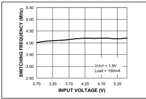
FIGURE 2-8: Input Voltage.
