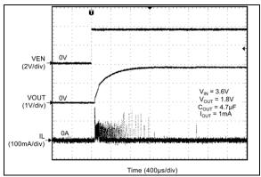
FIGURE 2-19: Start-Up,  $(I_{OUT} = 1 \text{ mA})$ .
