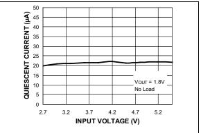
FIGURE 2-6: Quiescent Current vs. Input Voltage.
