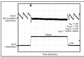
FIGURE 2-20: Load Transient, (1 mA to 150 mA).
