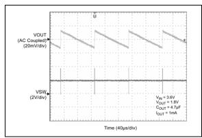
**FIGURE 2-13:** Switching Waveforms,  $(I_{OUT} = 10 \text{ mA}).$
