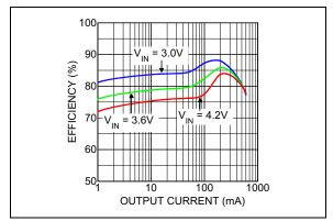
FIGURE 5-1: Efficiency under Load.
