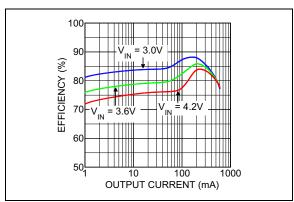
**FIGURE 2-2:** Efficiency  $(V_{OUT} = 1.8V)$ .
