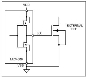
FIGURE 6-1: Low-Side Driver Block Diagram.
