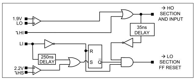
FIGURE 5-2: Input Logic Block in Figure 5-1.
