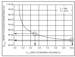
FIGURE 6-4:  $MOSFET R_{DS(ON)} vs. V_{GS}$ .
