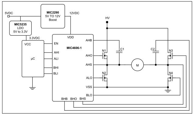
FIGURE 7-10: Full-Bridge DC Motor.
