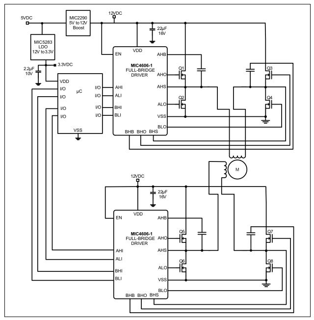
FIGURE 7-9: Stepper Motor Driver.
