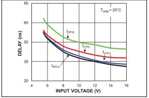
FIGURE 3-5: Propagation Delay vs. Input Voltage.
