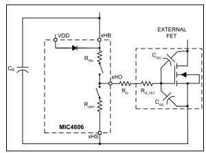
FIGURE 7-7: MIC4606 Driving an External High-Side MOSFET.
