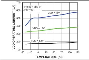
**FIGURE 3-8:** V<sub>DD</sub> Operating Current vs. Temperature.
