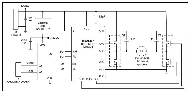
FIGURE 7-2: Door Lock/Unlock Circuit.
