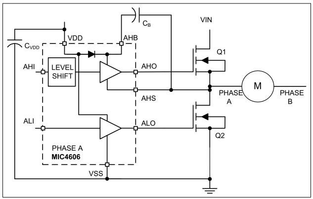
FIGURE 6-3: MIC4606 Motor Driver Example.
