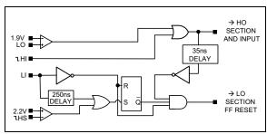
**FIGURE 7-3:** Adaptive Dead-Time Logic Diagram.
