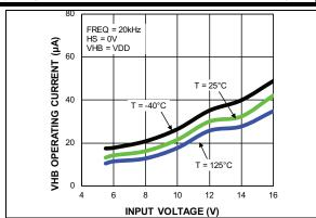
FIGURE 3-4: Input Voltage.
