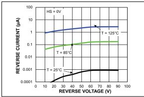
FIGURE 3-19: Bootstrap Diode Reverse Current.
