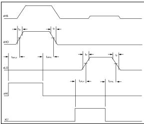
FIGURE 2-1: Separate Non-Overlapping LI/HI Input Mode (MIC4606-1)
