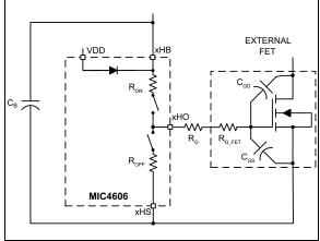
**FIGURE 7-1:** MIC4606 Driving an External MOSFET.
